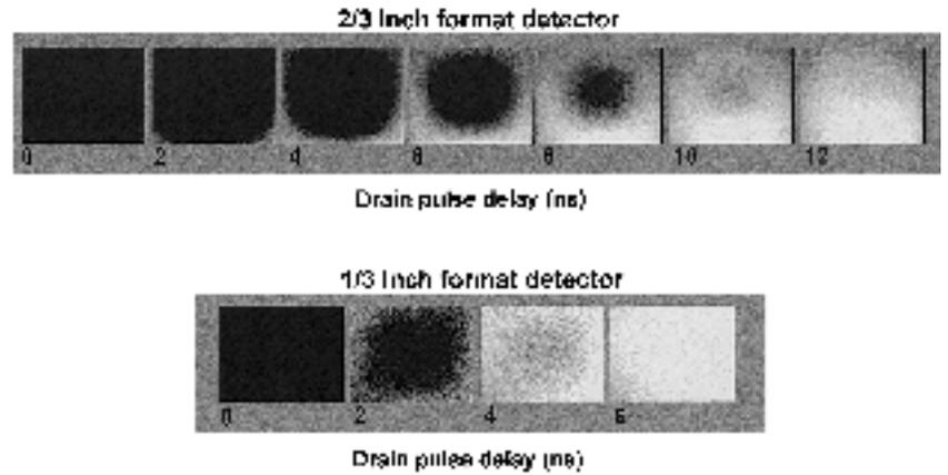
Fig. 2. Time gating response of interline transfer CCD detectors to a 4 ns FWHM pulsed blue LED.
