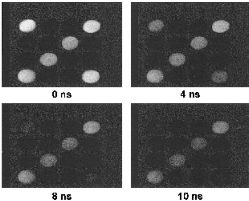
Fig. 5. Time-resolved imaging of fluorescent dyes using pulsed laser excitation and gated CCD detection.
