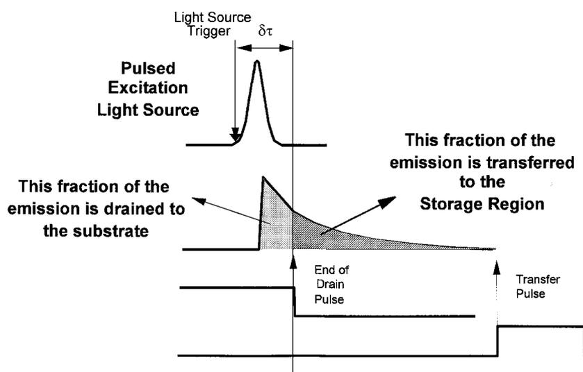
Fig. 1. Timing diagram for collection of time-resolved image.
