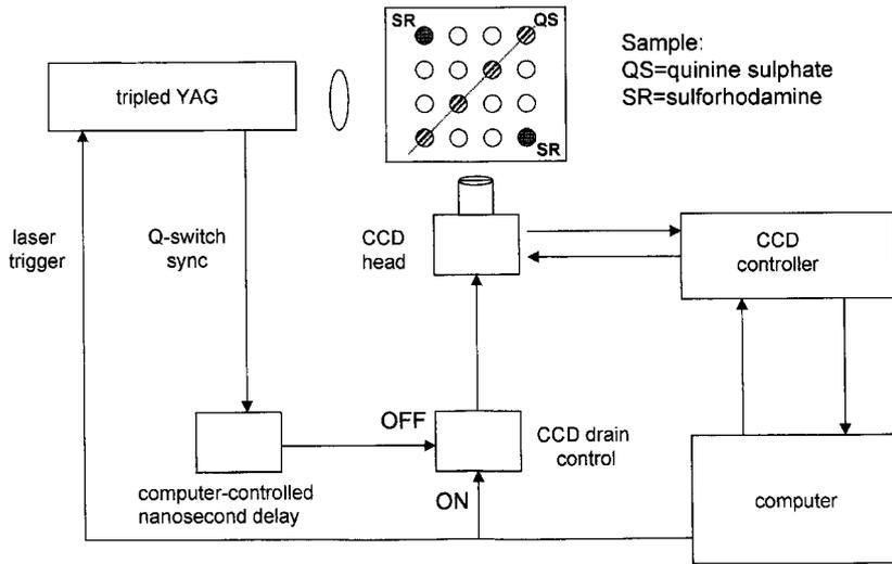
Fig. 4. Example of nanosecond time-resolved imaging using CCD with a pulsed Nd-YAG laser source.
