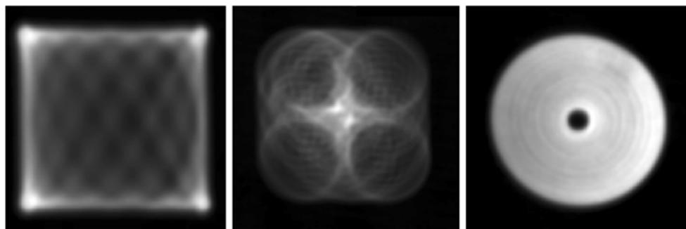
**Fig. 2** Laser scanning patterns: Lissajous figure (left), Lissajous figure superimposed on a circle (center), and an expanding/collapsing spiral (right). Clearly, the spiral pattern provides the most uniform coverage,
