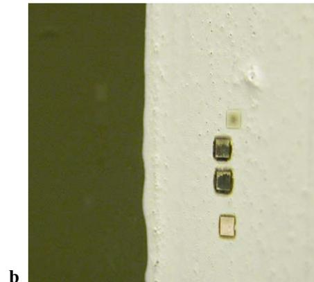
**Fig. 4** Ablation of paint using 515 nm 500 fs laser pulses with various scanning speeds of 1 shots per spot (*top pattern* in (**b**)), 10 shot/spot (*bottom pattern*), and 100 shot/spot (*two middle patterns*). Ablated vapor (**a**) and re-deposition of debris (**b**) can be clearly seen at the edges of the treated areas at the scanning speed of 10 shots/spot and 100 shots/spot
