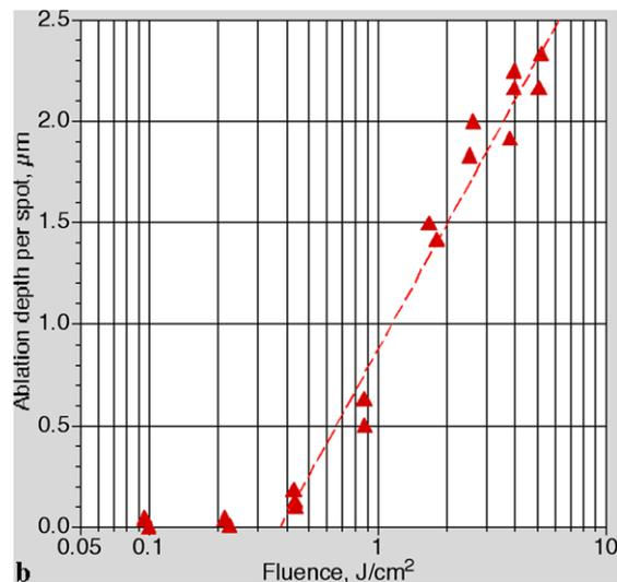
**Fig. 3** Racetrack scanning patterns (**a**) at various laser fluences from 0.09 to 5.2 J/cm<sup>2</sup> (the numbers under the patterns are fluences in J/cm<sup>2</sup>); and the ablation rate (**b**) of paint with 532 nm 1.5 MHz laser scanning with a speed of 10 m/s or 3 shots per spot
