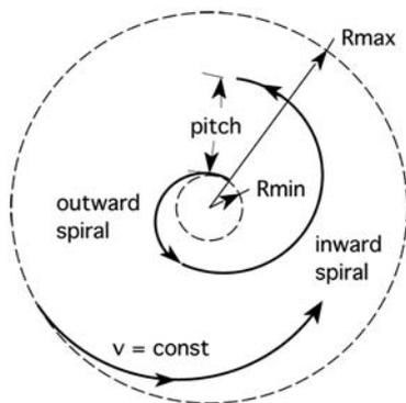
**Fig. 1** Scheme for a constant scanning velocity alternating spiral pattern. This is the most suitable for fast scanning of the laser beam due to the absence of sharp turning points
