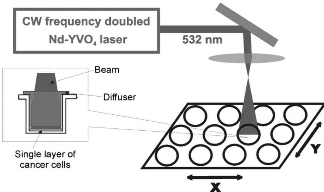
Fig. 1. The setting for laser irradiation of tumor cells. The beam from the laser (532 nm) was directed to the cell monolayer (without cell culture medium) passing through a lens and a diffuser to get flattened profile of ~4 mm diameter.
