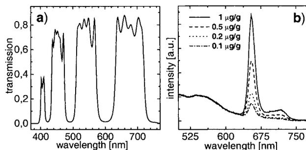
**Figure 3.** (a) Transmission of the triple band-pass filter XB29. (b) Emission of the fluorescence phantom with various mTHPC concentration levels after blue-light excitation (Wolf Combilight).
