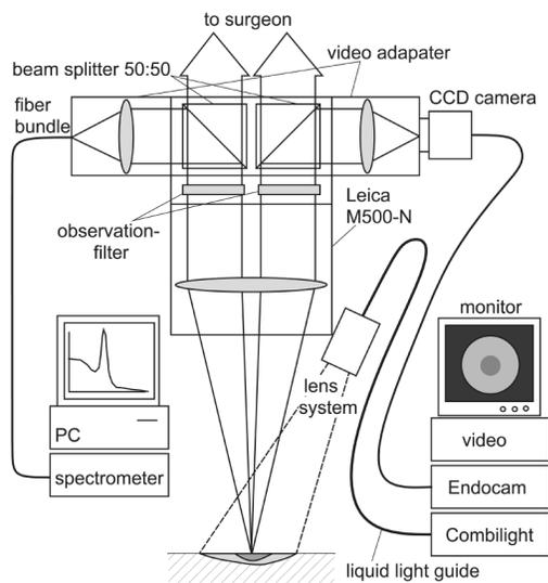
**Figure 2.** Modifications of the neurosurgical microscope (Leica M500-N) for mTHPC-mediated FGR and video-assisted diagnosis (Wolf). Blue excitation light is delivered by a liquid light guide to a lens system that is mounted beside the optical carrier of the microscope. An observation filter for the surgeon and the CCD camera is introduced in the optical path. Local spectral information can be obtained by a fiber-coupled sensitive spectrometer from the center part of the image.
