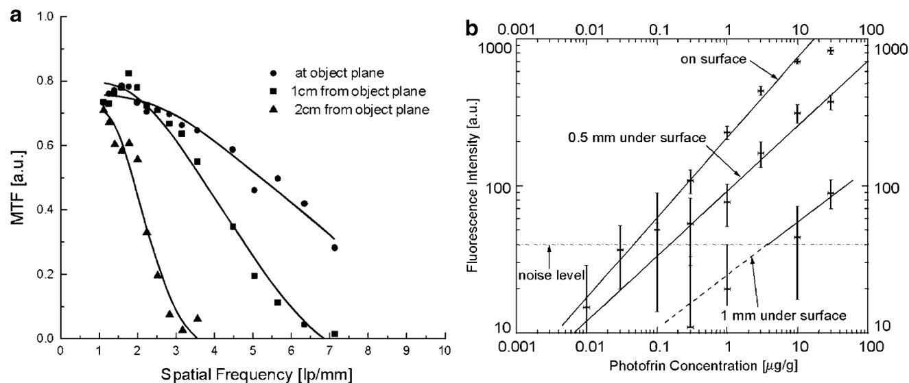
Fig. 4. Performance measurements. **a**: Fluorescence modulation transfer function measured with the resolution target placed at different distances from the focal plane in air. The solid curves are Gaussian fits to the experimental data points. Within the depth of focus ( $\pm 1$  cm), the MTF was  $> 10\%$  at 6.5
