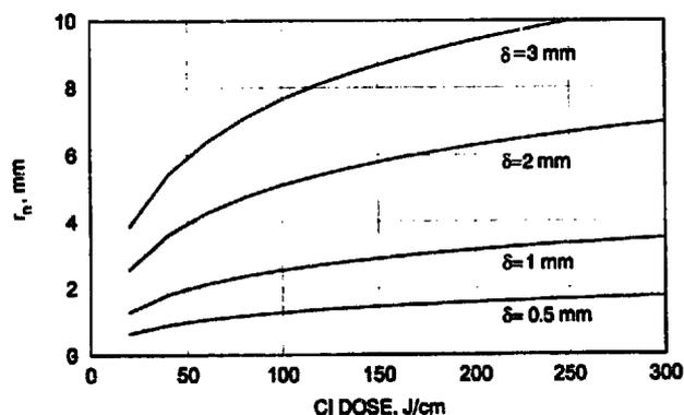
Fig. 4. Cylindrical insertion light delivery with PF at standard conditions. Dependence of necrosis radius ( $r_n$ ) on CI dose at different  $\delta$ .
