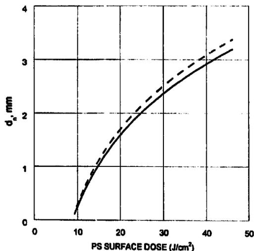
Fig. 2. Point surface light delivery with PF at standard conditions. Dependence of  $d_n$  on the total surface dose including scattered light. The assumed cavity volume is  $300 \text{ cm}^3$  and  $\delta = 2.0 \text{ mm}$ : solid line, calculated for PS delivery; dashed line, calculated for FS delivery.
