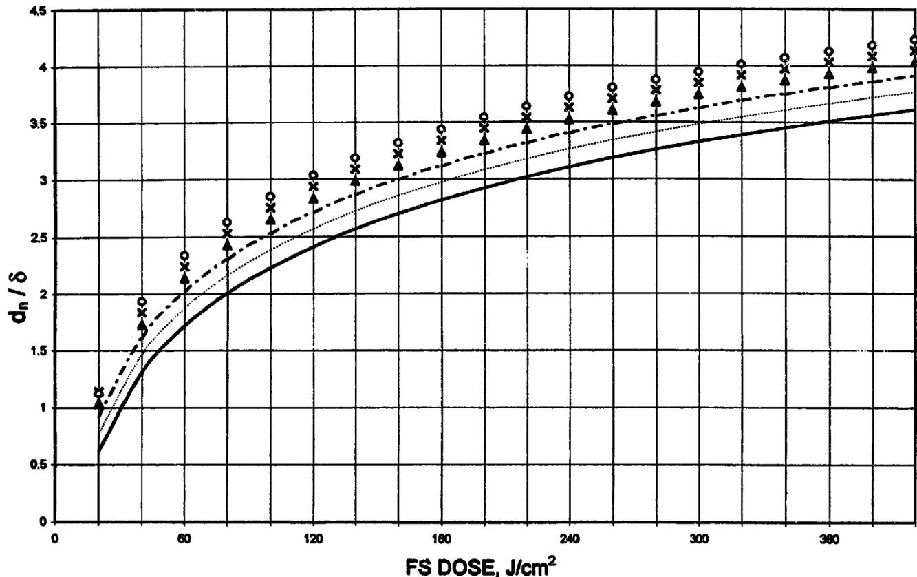
Fig. 1. Front surface light delivery with PF at standard conditions. Dependence of scaled necrosis depth ( $d_n/\delta$ ) on FS dose and diffuse reflectivity ( $R_n$ ): —  $R_n = 0.1$ ; ···  $R_n = 0.2$ ; - - -  $R_n = 0.3$ ; ▲  $R_n = 0.4$ ; x  $R_n = 0.5$ ; ○  $R_n = 0.6$ .
