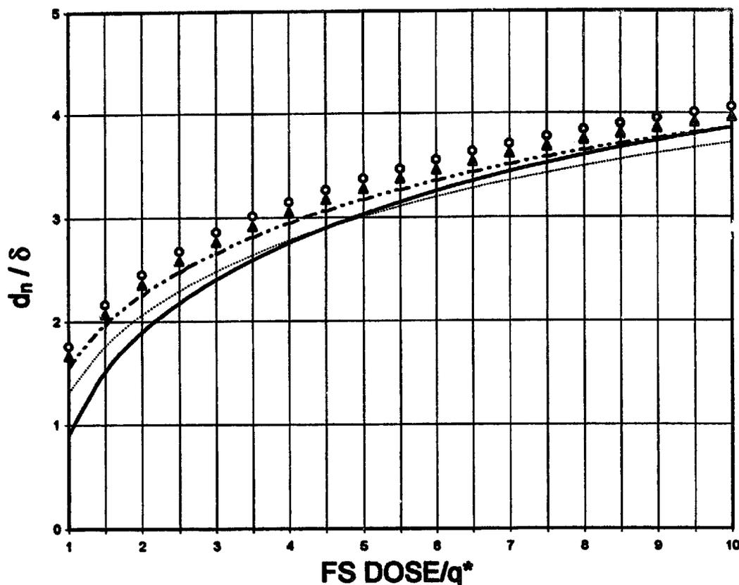
Fig. 5. Generalized front surface light dosimetry. Dependence of  $d_n/\delta$  on  $(E_0 t)/q^*$  for: —  $R_n=0.1$ ;  $\cdots$   $R_n=0.2$ ;  $-\cdot-$   $R_n=0.3$ ;  $\blacktriangle$   $R_n=0.4$ ;  $\times$   $R_n=0.5$ ;  $\circ$   $R_n=0.6$ . Based on Eq. (A6).
