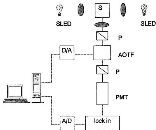
FIG. 2. Schematic diagram of the SLEDs AOTF fluorimeter: SLED, superluminescent light-emitting diode; S, sample; L, lens; P, polarizer; AOTF, acousto-optic tunable filter; PMT, photomultiplier tube; lock in, lock-in amplifier.
