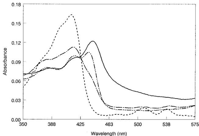
FIG. 3. Absorption spectra of  $1.0 \times 10^{-5}$  M Chl *a* in different media: 9:1 (v/v) acetone/water mixture (—);  $5.2 \times 10^{-2}$  M Brij-35 (---);  $8.8 \times 10^{-2}$  M SDS (- · - ·); and  $8.0 \times 10^{-2}$  M CTAB (· · · ·).
