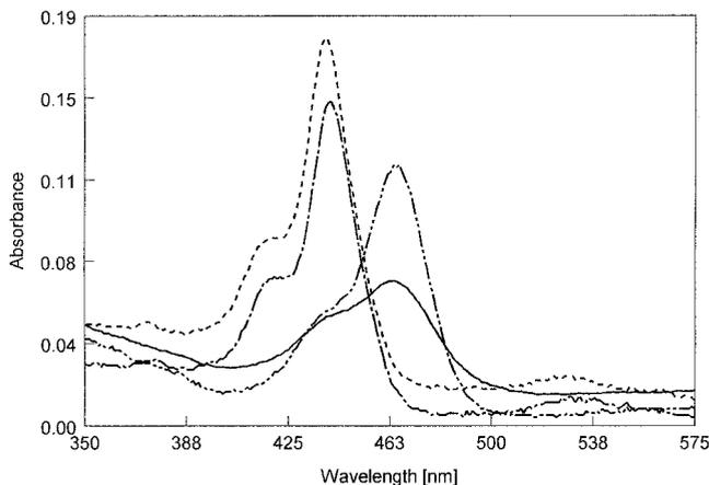
FIG. 4. Absorption spectra of  $1.0 \times 10^{-6}$  M Chl *b* in different media: 9:1 (v/v) acetone/water mixture (—);  $5.2 \times 10^{-2}$  M Brij-35 (---);  $8.8 \times 10^{-2}$  M SDS (- · - ·); and  $8.0 \times 10^{-2}$  M CTAB (· · · ·).
