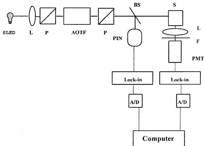
FIG. 6. Schematic diagram of the SLED AOTF fluorimeter for excitation-spectra measurements: SLED, superluminescent light-emitting diode; S, sample; L, lens; P, polarizer; AOTF, acousto-optic tunable filter; PMT, photomultiplier tube; lock-in, lock-in amplifier; PIN, photodiode.
