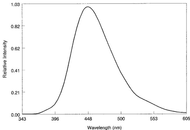
FIG. 1. Spectral output intensity of the superluminescent bright-blue light-emitting diode.
