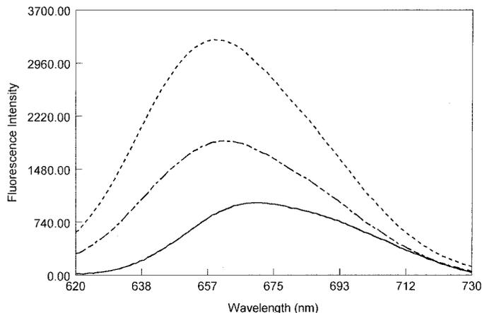
FIG. 5. Fluorescence spectra of  $1.10 \times 10^{-6}$  M Chl *a* (—);  $1.10 \times 10^{-6}$  M Chl *b* (---); and a mixture of  $5.50 \times 10^{-7}$  M Chl *a* and  $5.50 \times 10^{-7}$  M Chl *b* (- · - ·) in  $8.0 \times 10^{-2}$  M CTAB.
