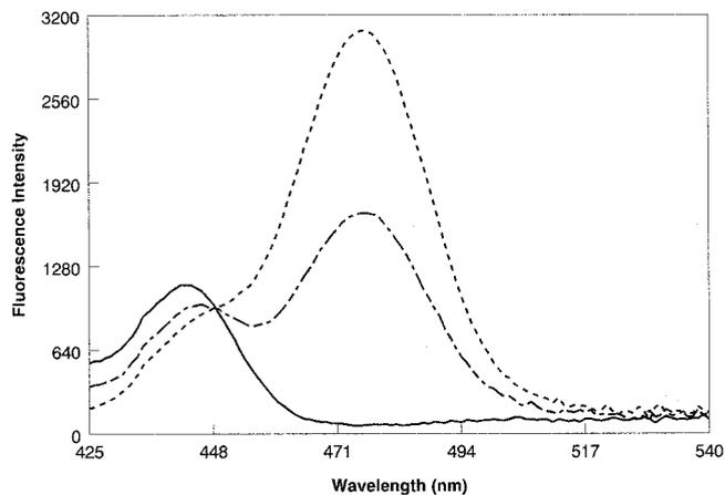
Fig. 7. Excitation spectra of  $1.10 \times 10^{-6}$  M Chl *a* (—);  $1.10 \times 10^{-6}$  M Chl *b* (---); and a mixture of  $5.50 \times 10^{-7}$  M Chl *a* and  $5.50 \times 10^{-7}$  M Chl *b* (- - -) in  $8.0 \times 10^{-2}$  M CTAB.
