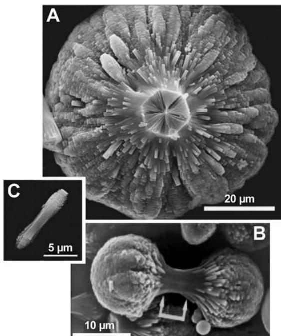
**Fig. 1.7** Scanning electron micrographs showing fractal pattern formation by hierarchical growth of fluorapatite–gelatin nanocomposites: (A) half of a dumbbell aggregate viewed along the central seed axis, (B) dumbbell aggregate at an intermediate growth state, and (C) central seed exhibiting tendencies of splitting at both ends (“small” dumbbell). Adapted from [119], reproduced by permission of Wiley-VCH.
