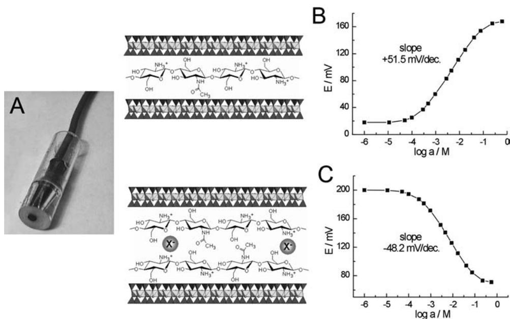
**Fig. 1.8** (A) Design of a chitosan-montmorillonite sensor. Arrangement of chitosan chains in the clay interlayer space as a monolayer (B) or a bilayer (C) resulting in opposite behavior when measuring NaCl solutions of increasing concentration by direct potentiometry.
