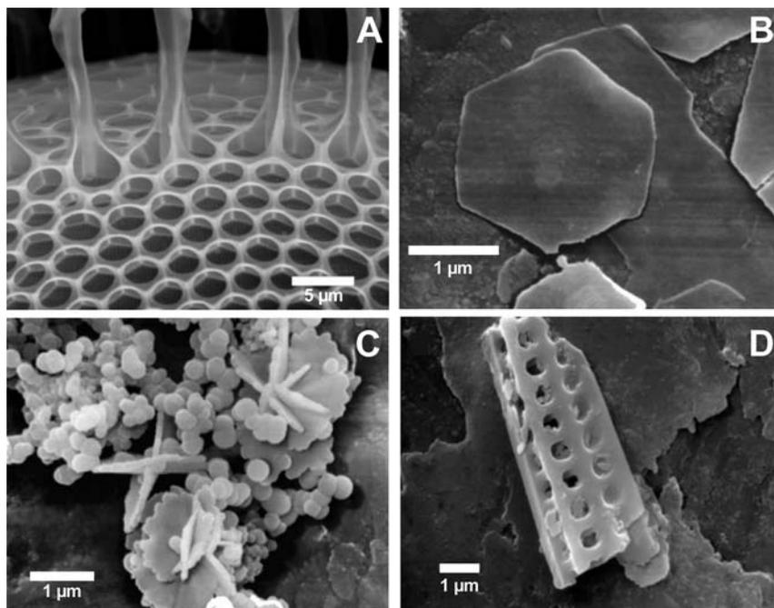
**Fig. 1.2** Scanning electron micrographs of (A) the silica wall of the diatom *Stephanopyxis turris* (reproduced from [21] by permission of Wiley-VCH) and (B–D) singular morphologies of silica synthesized using poly-L-lysine and pre-hydrolyzed tetramethyl orthosilicate (TMOS) under different experimental conditions: (B) unperturbed solution, (C) flowed through a 1/8" I.D. tube and (D) stirred for 25 min. Reproduced from [39] by permission of The Royal Society of Chemistry.
