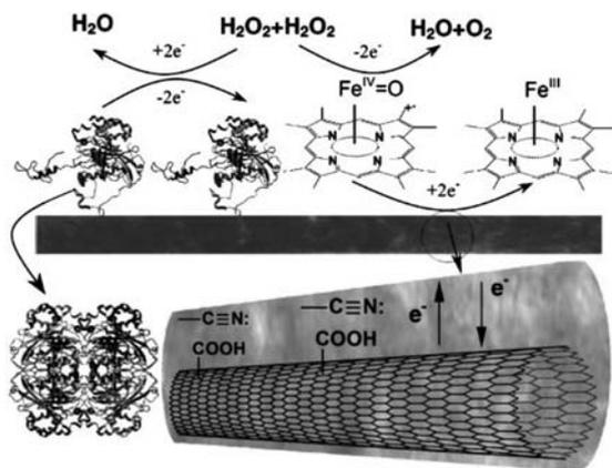
**Fig. 1.16** Schematic representation of the nanofibrous poly(acrylonitrile-*co*-acrylic acid) membrane containing MWCNTs, as well as the promoted electron transfer from hydrogen peroxide to the immobilized catalase through the PANCAA/MWCNTs nanofiber. Reprinted from [209] (reproduced by permission of Wiley-VCH).
