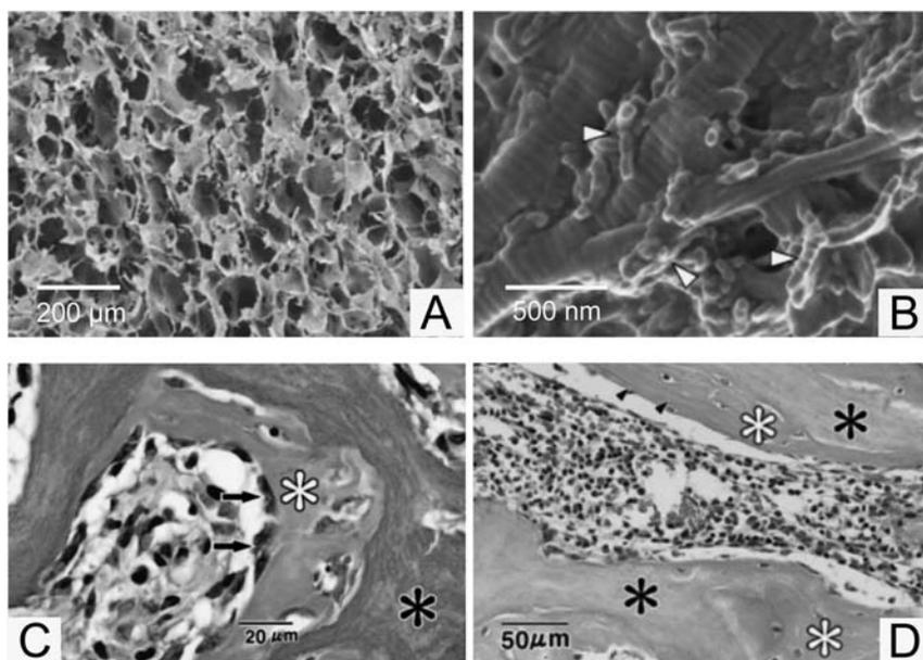
**Fig. 1.6** (A and B) Scanning electron micrographs of the porous hydroxyapatite–collagen nanocomposite scaffolds at different magnifications. Arrowheads in B indicate the hydroxyapatite nanocrystals on the collagen fibrils. Histology at (C) 1 week and (D) 4 weeks after
