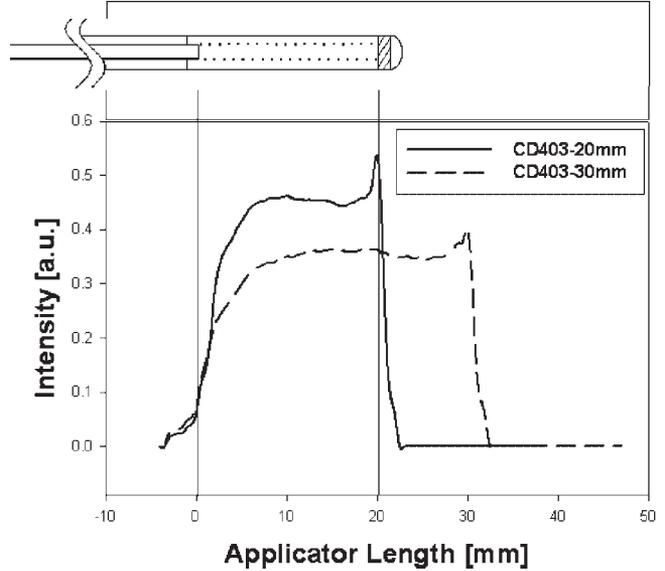
Fig. 1. Top: Cross section of the applicator CD403-20 including X-ray marker at the distal end. Bottom: Radiation profile of the two applicator types,  $l = 20$  mm (—) and  $l = 30$  mm (- - -).
