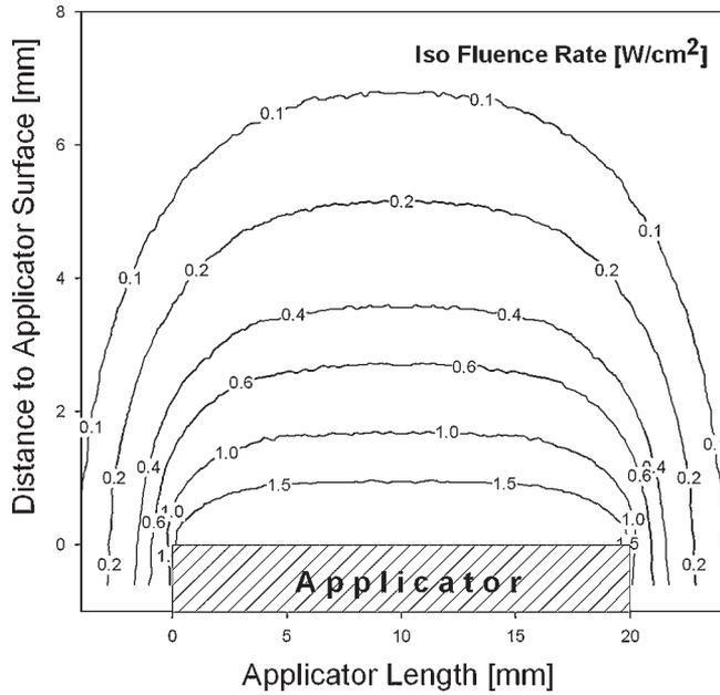
Fig. 3. Iso-fluence rates of a cylindrical light diffuser calculated by Monte-Carlo simulations.
