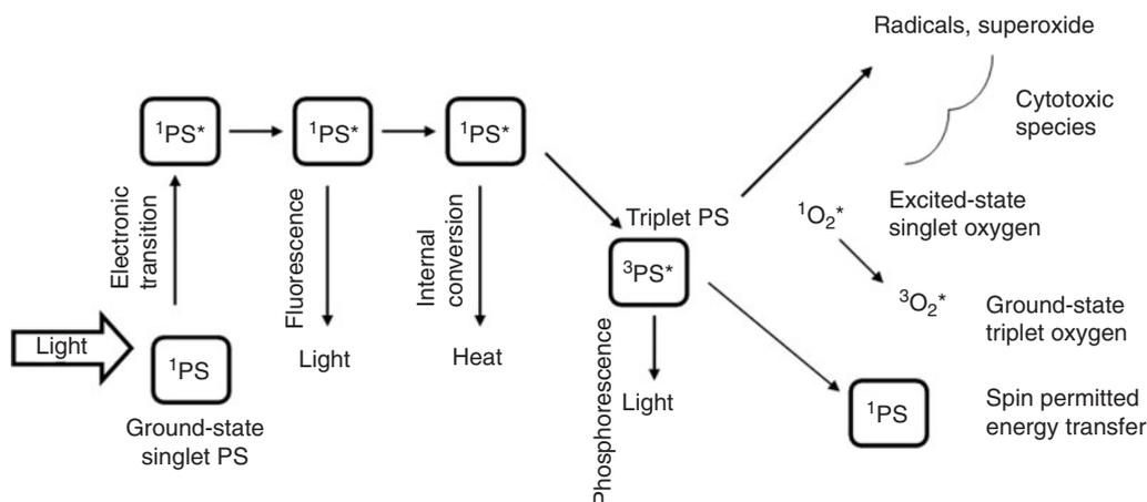
**Fig. 1.** Schematic representation of the photochemical process of excitation of the photosensitizer (PS), including the possibilities of luminescence (fluorescence and phosphorescence), the singlet and triplet excited states and the reactive oxygen species generated by the energy transfer from the PS.
